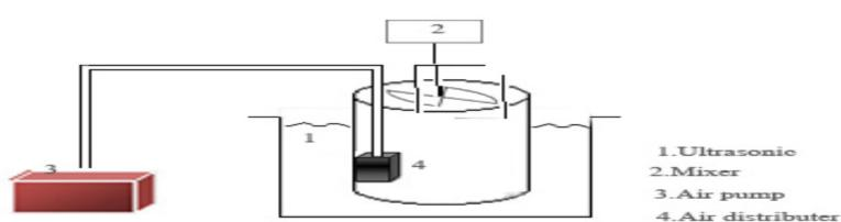
**Figure 1 Those of reactor Sonolysis**
