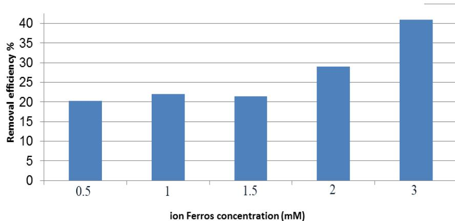
**Figure 4** Effect of ferrous ion concentration on color removal efficiency by sonolysis process in real textile wastewater (pH optimized 2-time of 240 minutes, the air flow rate of 1.5 liters per minute, a frequency of 28 kHz)
