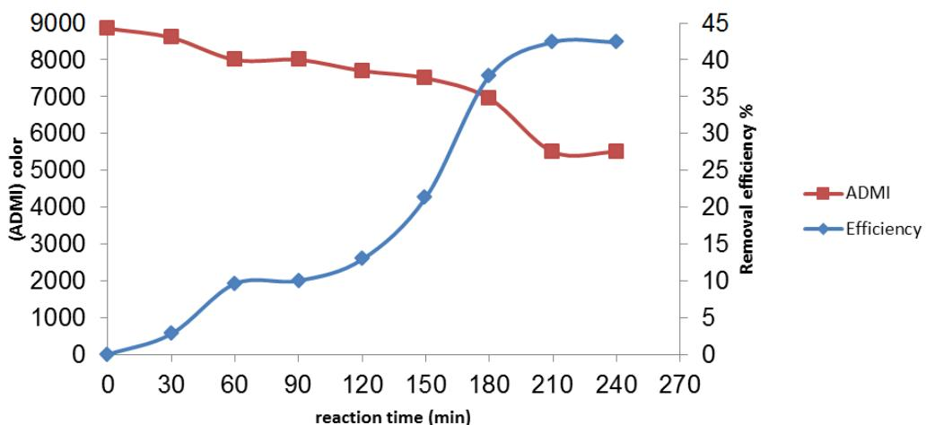
**Figure 6** Effect of reaction time on dye removal by actual of wastewater sonolysis process based on reactive dye in optimal conditions ( $2 = pH$ , ion concentration down to 3 mM, air flow rate of 1 liter per minute)
